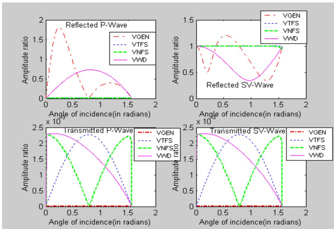
Figures 22-25. Variation of the amplitude ratios of reflected P-wave, reflected SV-wave, transmitted P-wave and transmitted SV-wave with angle of incidence of P-wave in case of elastic solid
