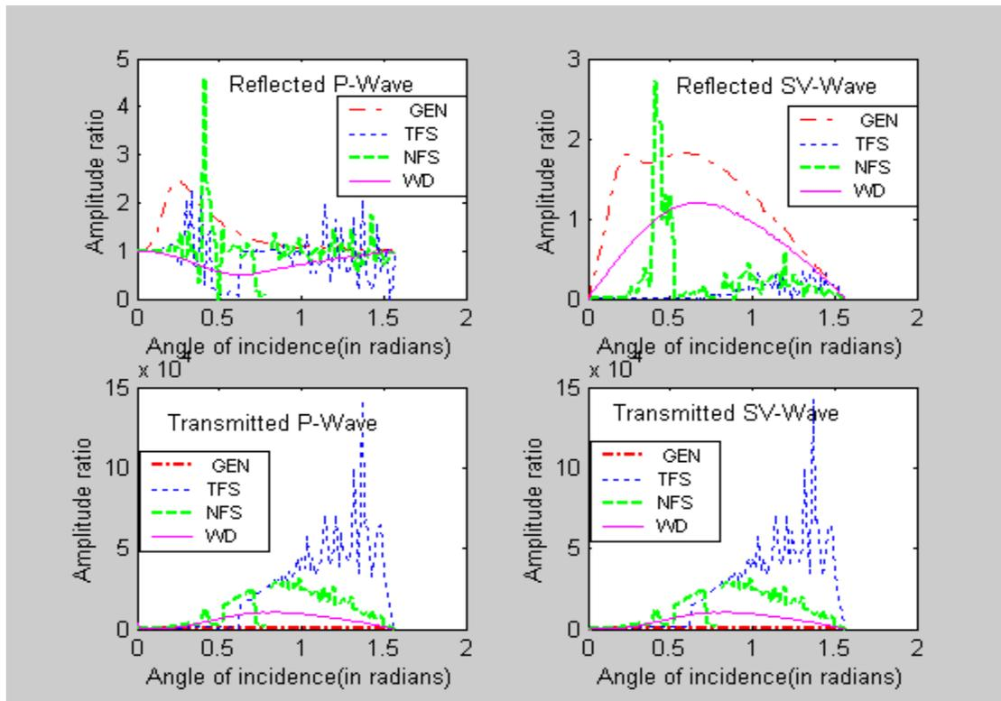
Figures 2-5. Variation of the amplitude ratios of reflected P-wave, reflected SV-wave, transmitted P-wave and transmitted SV-wave with angle of incidence of P-wave.
