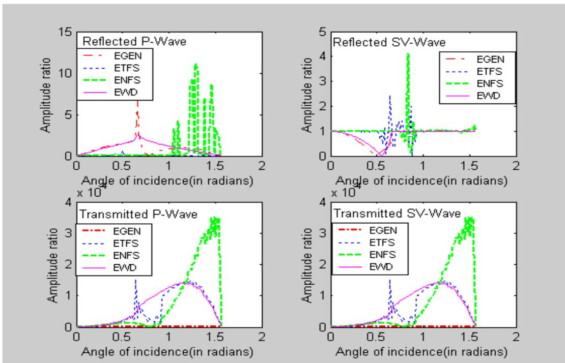
Figures 14-17. Variation of the amplitude ratios of reflected P-wave, reflected SV-wave, transmitted P-wave and transmitted SV-wave with angle of incidence of P-wave in case of empty porous solid.
