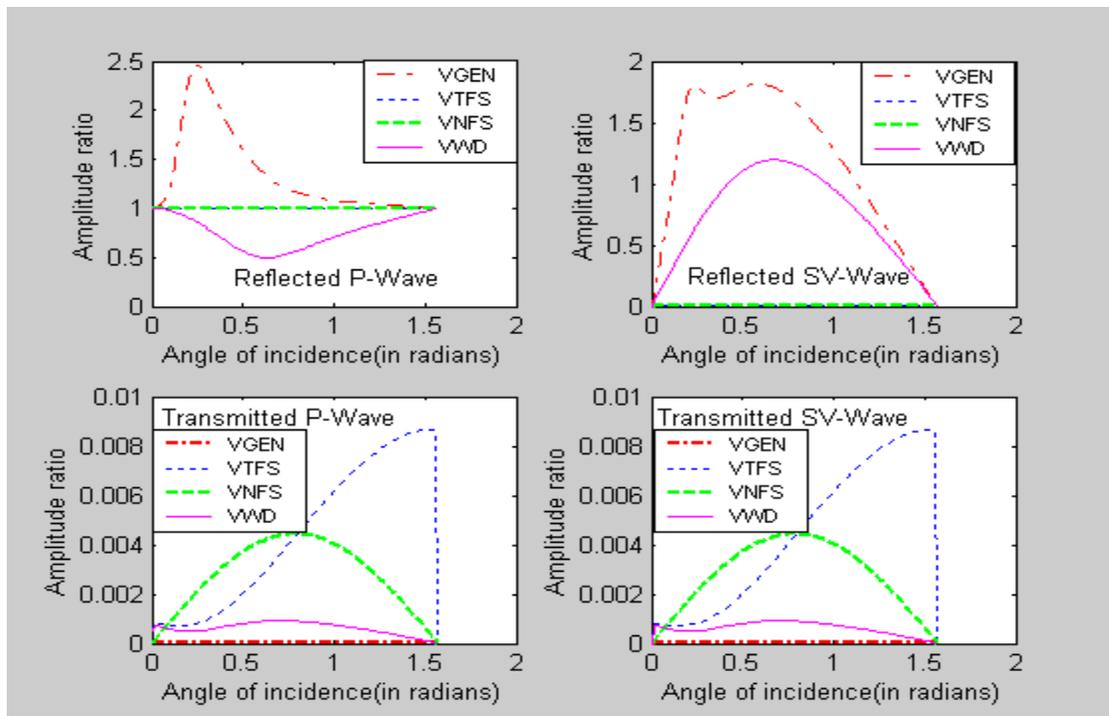
Figures 18-21. Variation of the amplitude ratios of reflected P-wave, reflected SV-wave, transmitted P-wave and transmitted SV-wave with angle of incidence of P-wave in case of elastic solid
