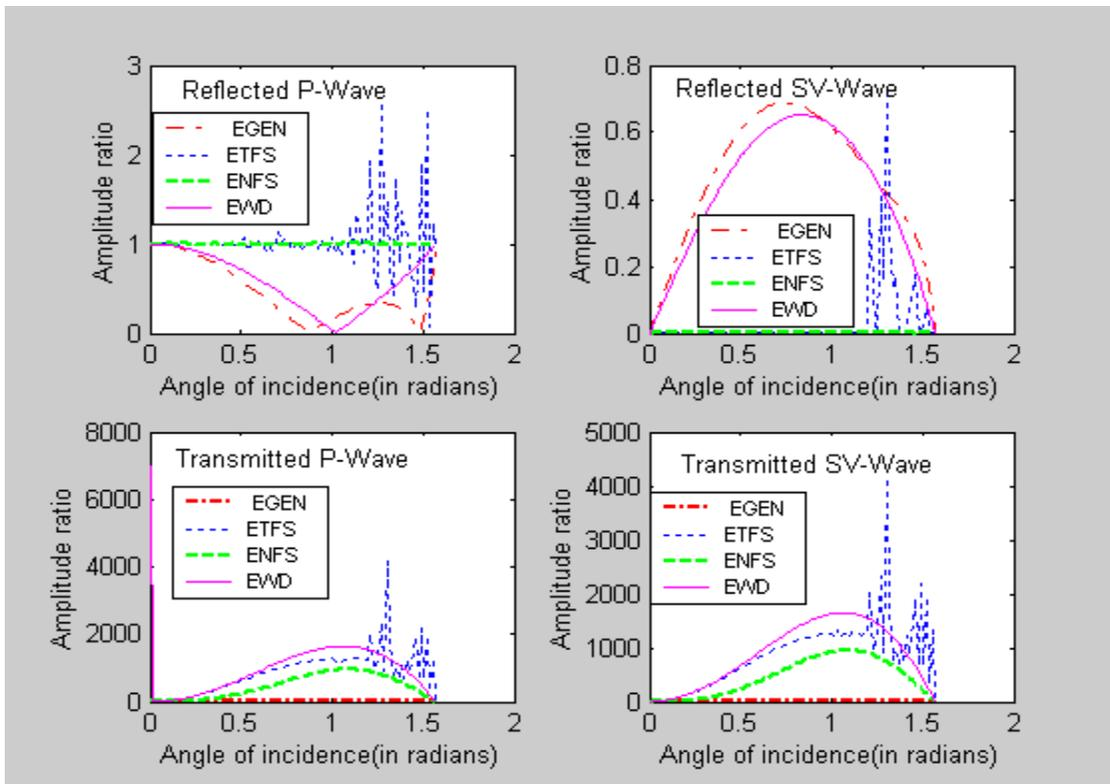
Figures 10-13. Variation of the amplitude ratios of reflected P-wave, reflected SV-wave, transmitted P-wave and transmitted SV-wave with angle of incidence of P-wave in case of empty porous solid.
